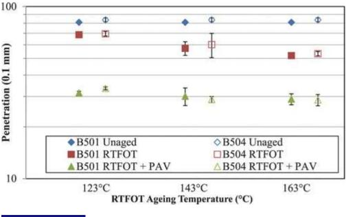
Figure 2. Penetration value as a function of RTFOT ageing temperature for bitumen B501 and B504.
